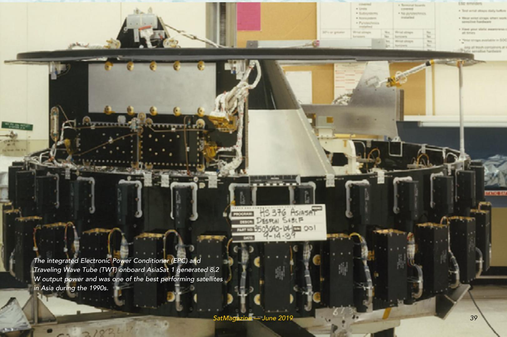
The integrated Electronic Power Conditioner (EPC) and Traveling Wave Tube (TWT) onboard AsiaSat 1 generated 8.2 W output power and was one of the best performing satellites in Asia during the 1990s.
