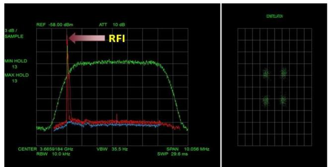
Fig. 4 Modulation Analysis of the carrier which was suffering from Interference B
